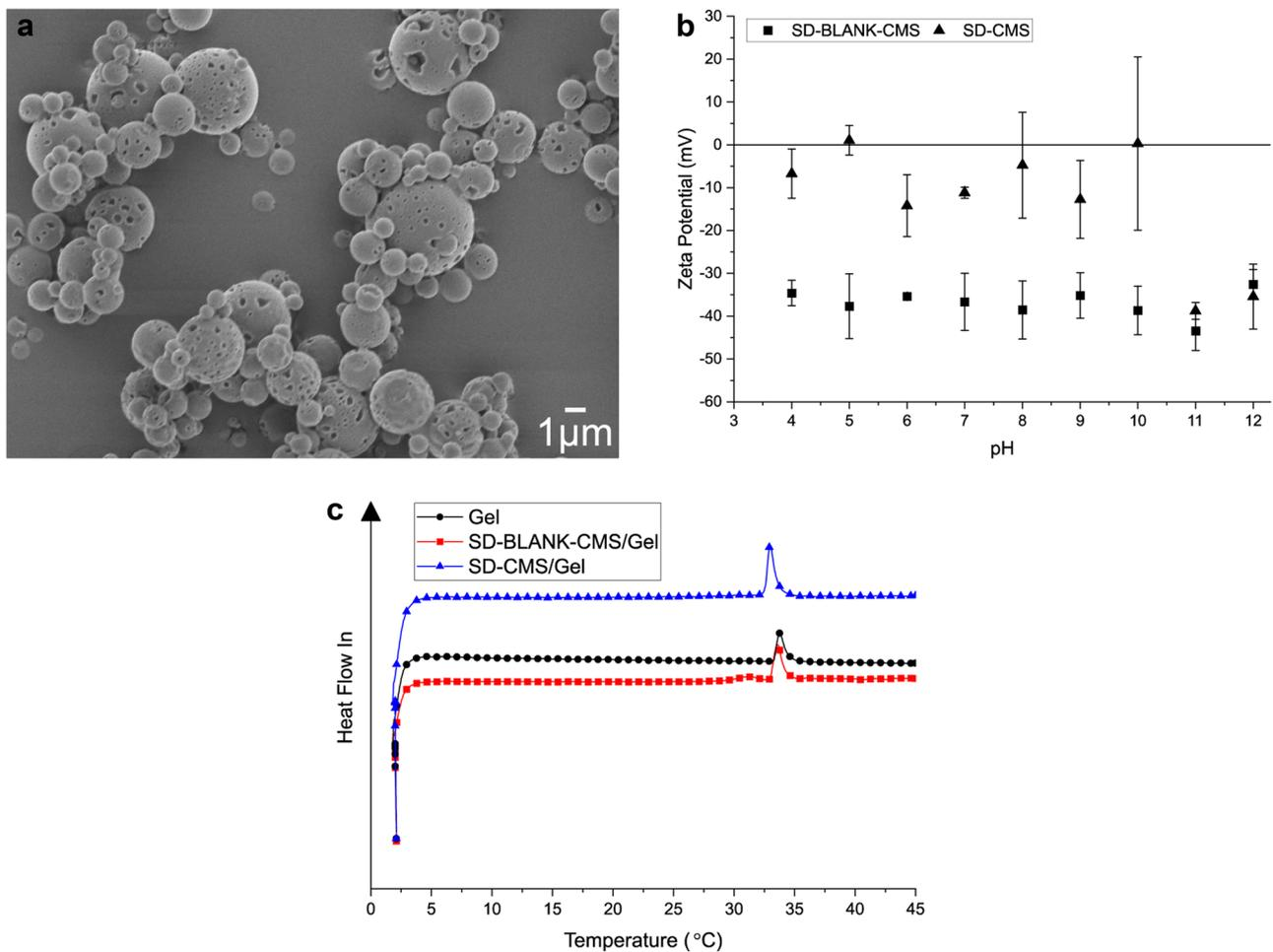
**Fig. 1** **a** Scanning electron microscopy (SEM) of SD-CMS, **b** Zeta potential of microsphere formulations, and **c** determination of lower critical solution temperature (LCST) via differential scanning calorimetry (DSC). LCST of SD-CMS/Gel decreased to 32 °C from the base Gel at 34 °C
