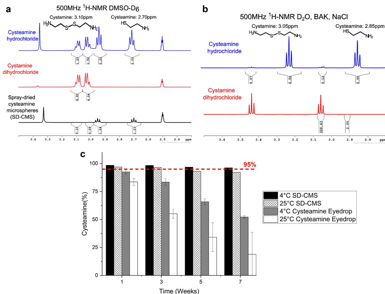
**Fig. 3** **a**  $^1\text{H-NMR}$  of cysteamine microspheres (SD-CMS) in deuterated dimethyl-sulfoxide (DMSO- $\text{D}_6$ ) with cysteamine (2.70 ppm) and cystamine (3.10 ppm) reference peaks. **b**  $^1\text{H-NMR}$  of cysteamine eyedrops with benzalkonium chloride (BAK) and sodium chloride (NaCl) in deuterated water ( $\text{D}_2\text{O}$ ) with cysteamine (2.85 ppm) and cysteam-
